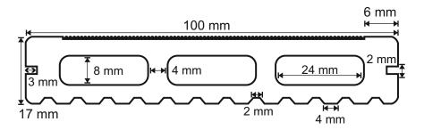
Type: Wood Plastic Composites Weight: 1.6 Kg Each Long Meter Polymer base: PVC (Ploy Vinyl Chloride) ASTM Standards:
