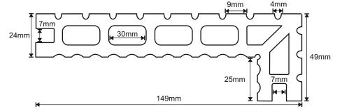
Type: Wood Plastic Composites Weight: 4 Kg Each Long Meter
