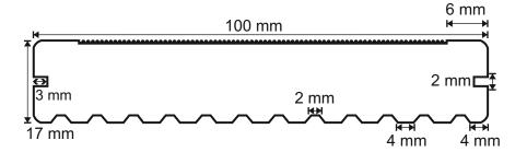
Type: Wood Plastic Composites Weight: 2.45 Kg Each Long Meter
