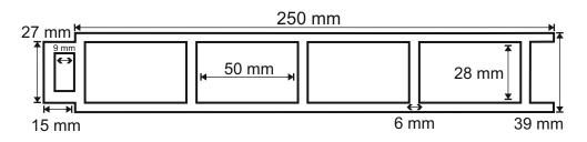
Type: Wood Plastic Composites Weight: 5.8 Kg Each Long Meter
