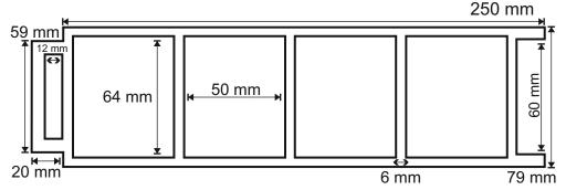
Type: Wood Plastic Composites Weight: 9 Kg Each Long Meter
